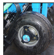
• Unit counter on wheel to check the surfaces worked
