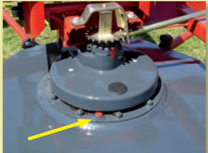
Meter cap for checking oil level in the camshaft mechanism.
