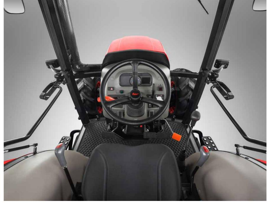
Wide doors allow the comfortable entry into the cab. The suspended seat, adjustable steering wheel and other ergonomic features ensure comfortable work.
