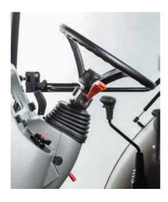
The HORTUS HS is equipped with a hydraulic reverser (PowerShuttle), which allows to conveniently change the driving direction without using the clutch pedal.
